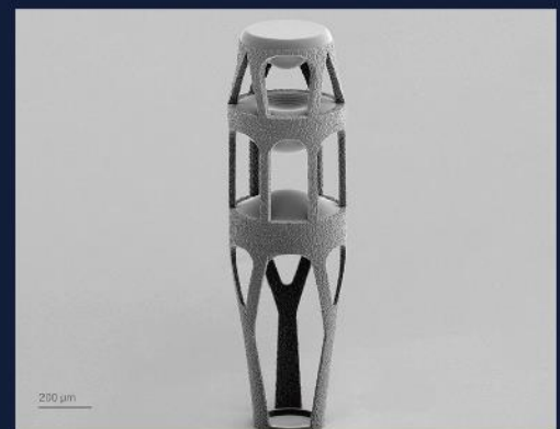
High-precision optics developed for a miniature endomicroscope. The stacked freeform lenses are 3D printed by 2GL.
